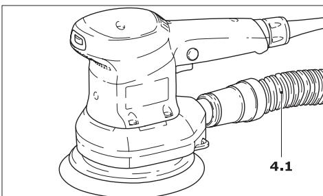
In order to avoid frequent changing of the turbo-filter when carrying longer sanding jobs, it is possible to connect a Festool extractor to the unit instead of using inbuilt extraction.
